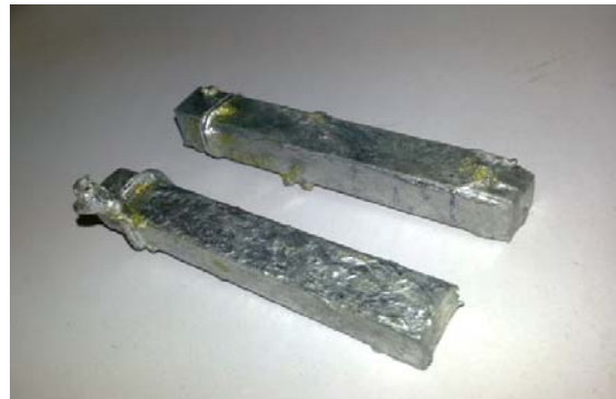
Figure 3 Hot Dip Galvanized samples of Mild Steel Grade 1014
