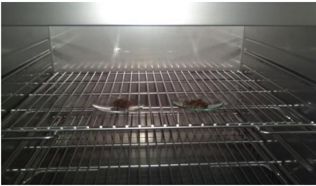
Figure.3. Testing of Moisture Content
