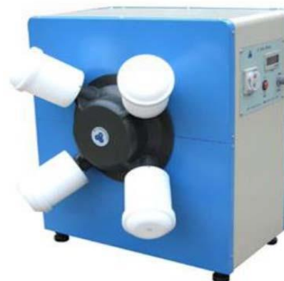
Figure 1: Mixer, used for powder mixing
