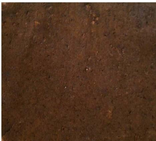
Figure 16: Stereograph of BaTiO 3 Pellet, Sintered at 1350°C, 7X Magnification
