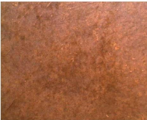
Figure 15: Stereograph of BaTiO 3 Pellet, Sintered at 1300°C, 7X Magnification
