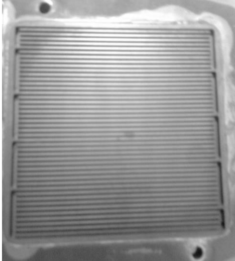
Figure 3. Gas flow channels engraved in bipolar plate
