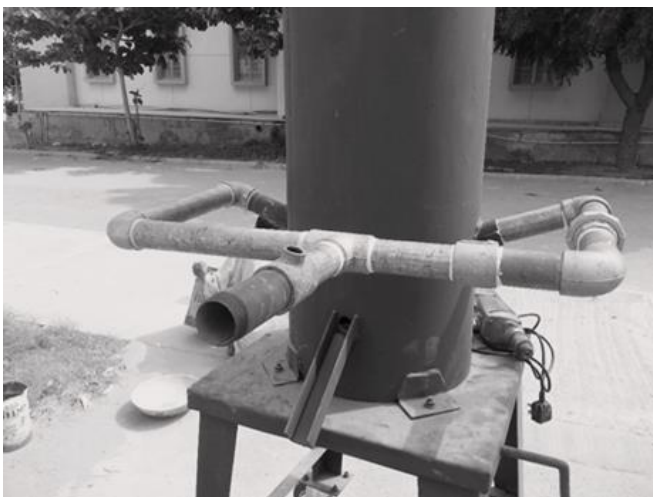
Figure 4: Angle tuyeres design used in structure
